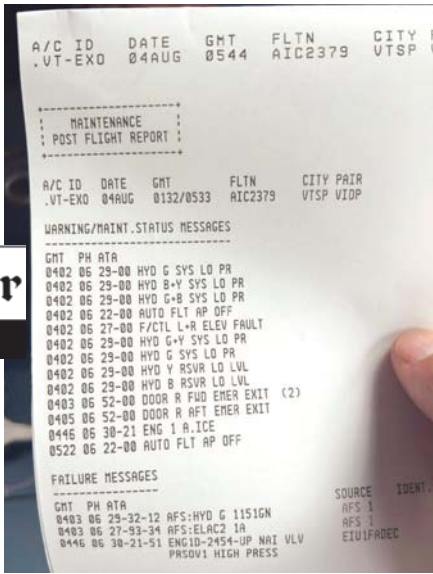
The aircraft’s post-flight maintenance on August 4 records low-pressure warnings involving all three hydraulic systems, an autopilot disconnect and an elevator flight-control fault around 04.02 UTC PIONEER PHOTO
